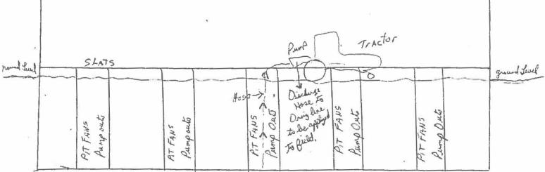
you back a tructor up to pump outs + put a pipe on how to bottom of pit and pump Manue out. This is the only way to get menure out of pit. Pits 1+2 due same demonsions + an the same.
